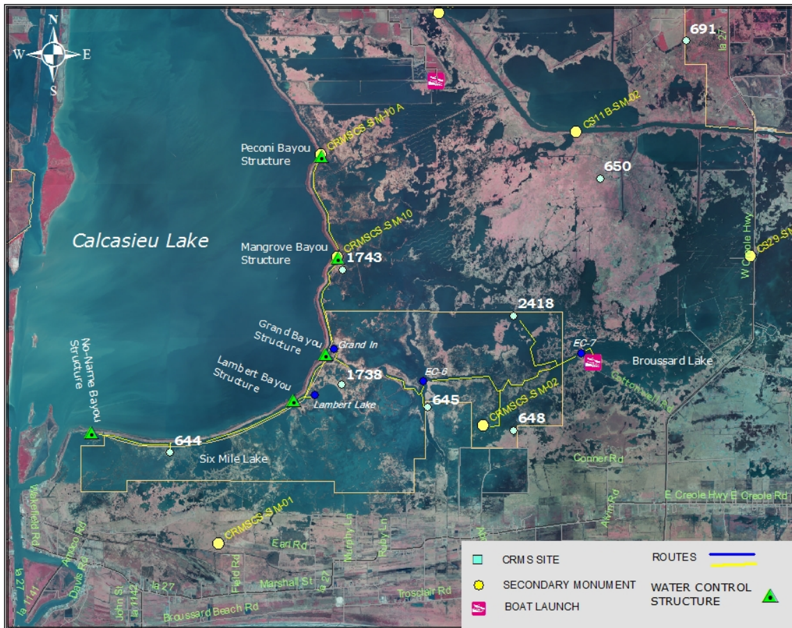
Figure 32. Southeastern marshes bayou structures monitored by CPRA in Calcasieu Lake. Map courtesy of CPRA.
