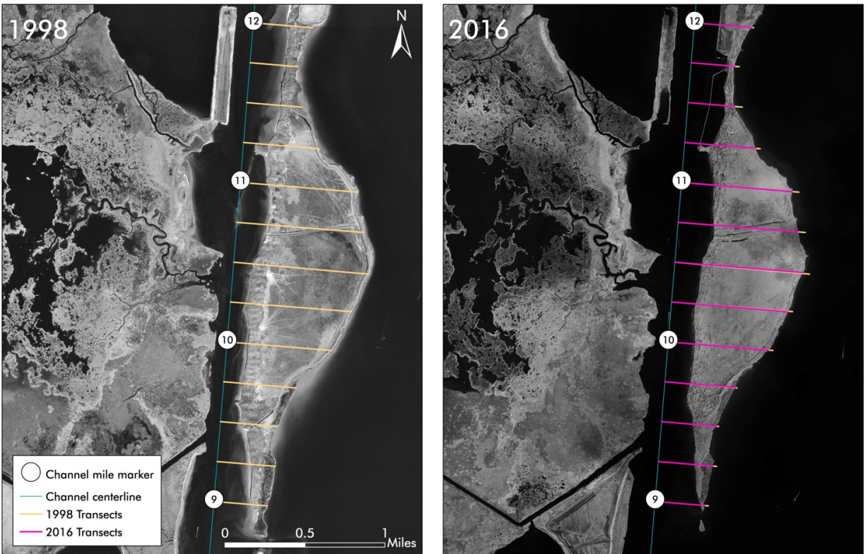
Figure 42. Transects from centerline to spoil bank shoreline facing Calcasieu Lake in 1998 (yellow) and 2016 (magenta) for river miles 9-12.
