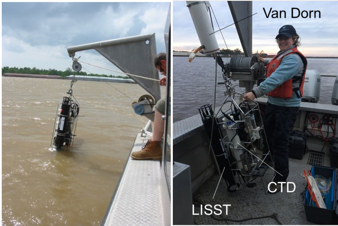
Figure 19. Photograph of a CTD/LISST cast at a transect station. Left, the casting instrument profiler is being deployed. Right, the LISST is attached to the CTD profiler frame and the Van Dorn sampler is attached above the frame.
