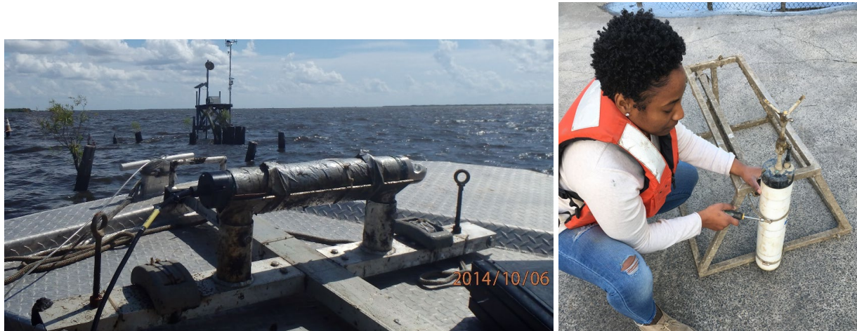
Figure 14. Photographs of current and wave instruments. Left, Aquadopp on sled mount resting on the vessel deck, right, ADV mounted on a bottom-deployed tripod.
