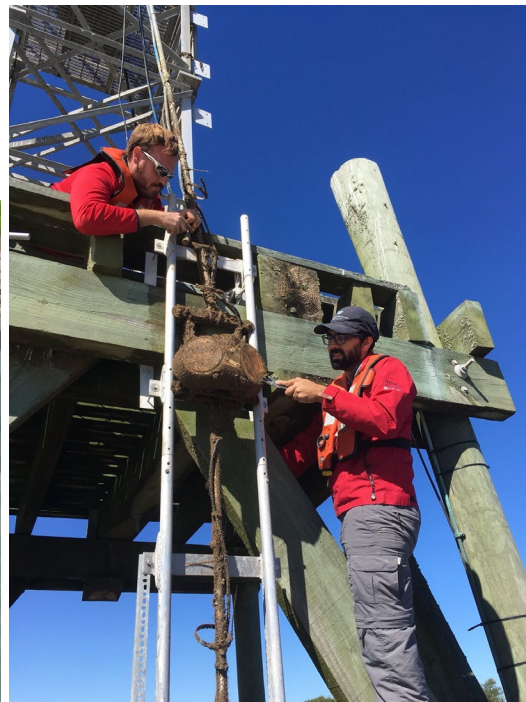
Figure 13. H-ADCP deployment. Left, visual schematic of a deployed H-ADCP where the two acoustic transducers record water velocities at one fixed depth (image from Sontek: http://www.sontek.com/productsdetail.php?SonTek-SL-8 ). Right, Institute employees service and clean one of the bio-fouled H-ADCPs at SCC.
